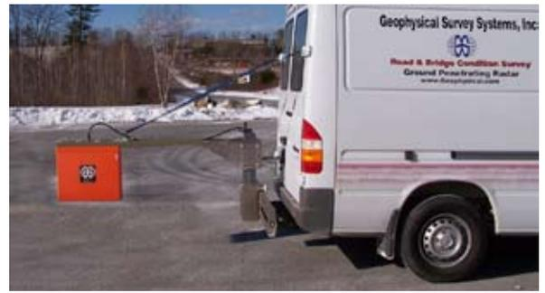
GSSI 1 GHz (Model 4108) horn antenna for high-speed road surveys.
