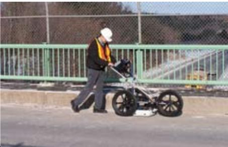
Bridge deck survey conducted with 1.6 GHz (Model 5100) antenna.
