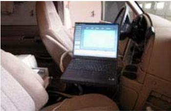
The JILS-20T-FWD is a truck (Ford F350 XLT or equivalent) mounted FWD, which is operated from the driver seat in the vehicle. The data from the tests are displayed on a cab-mounted laptop computer and recorded for future analysis.
