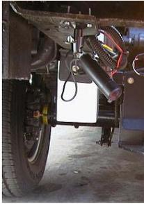
For vehicle positioning and joint testing, a color video monitoring system from Accele Vision (<http://www.accele.com>) is included in the base price. A flip down video monitor that saves space and color video camera are mounted for efficient tow vehicle positioning for test location load transfer testing and monitoring.
