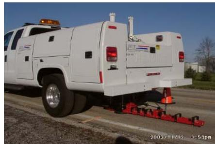
Therefore, ARA narrowed the choices down to Dynatest and JILS. ARA conducted side-by-side testing on three different pavement structures for a comparison of load pulses, deflection basins, and back calculated sub grade moduli. In addition, equipment characteristics of both machines were analyzed based on the following criteria:
