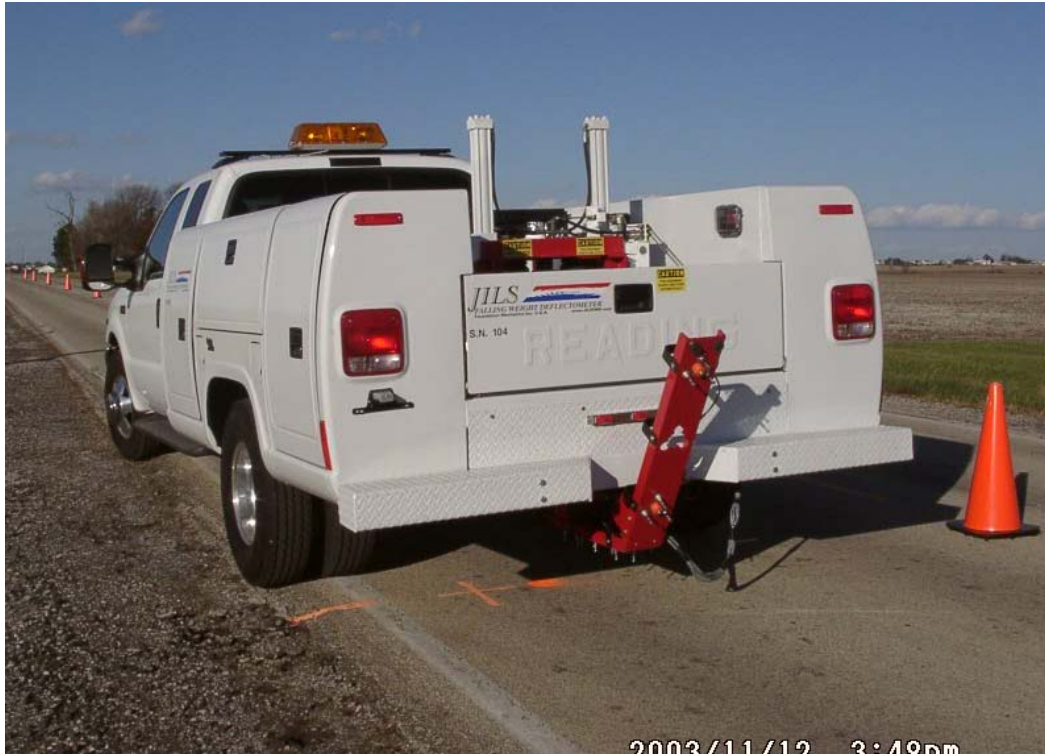
Figure 1. JILS Model 20T FWD with the sensor bar in the transport position.
