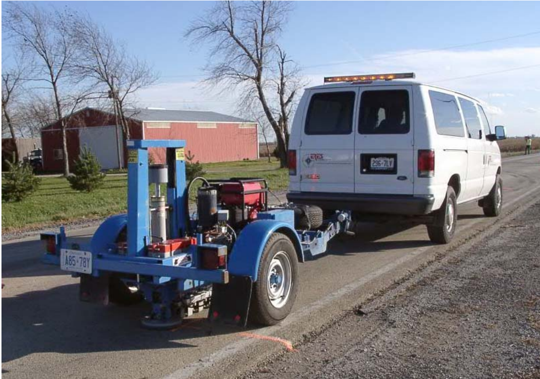
Figure 3. Dynatest Model 8002 FWD with the load plate in the testing position.
