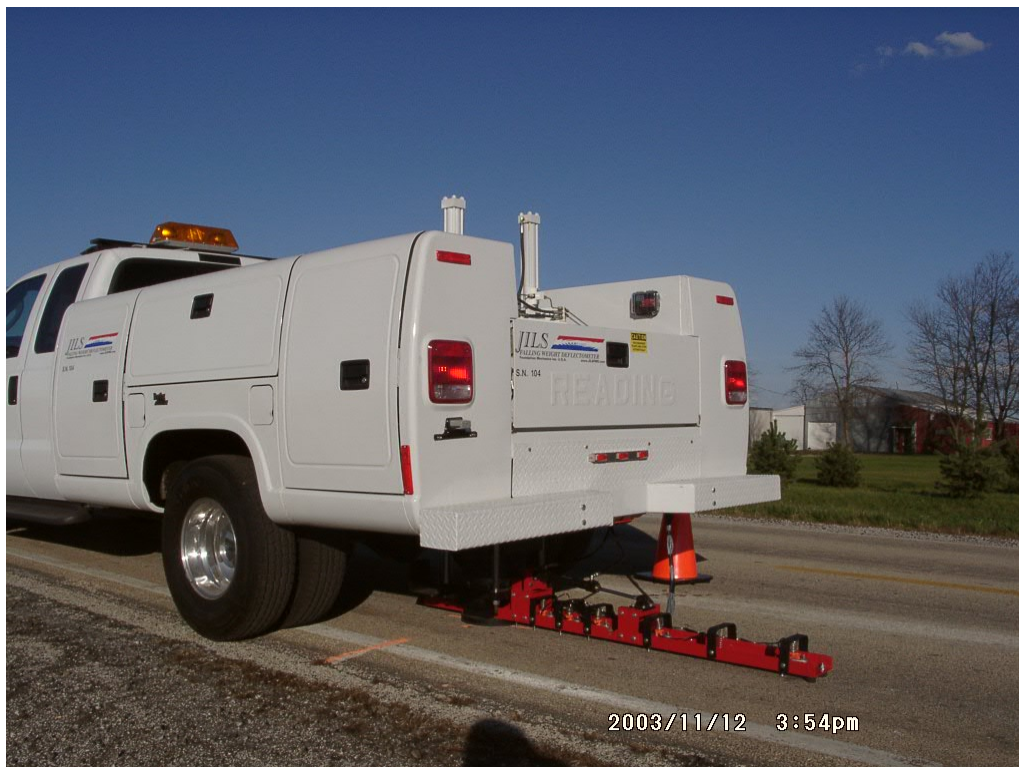
Figure 2. JILS Model 20T FWD with sensor bar in the testing position.
